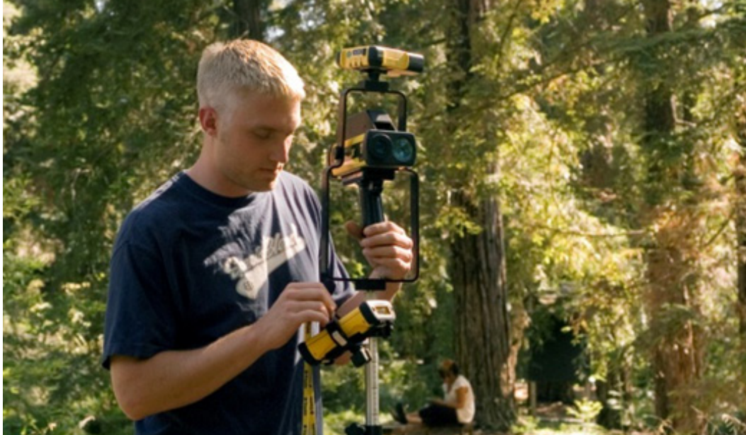
Figure 7.8. GPS Data Collection with a Laser Rangefinder
